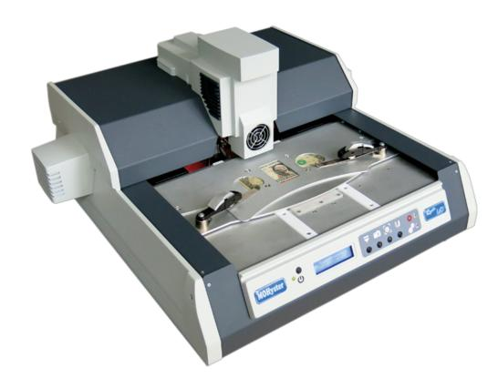
MOHyster Regula 7708 is specifically designed to be used in applied research, particularly for the development of new and improvement of currently existing document security features with magnetic properties. The solution is also perfect for monitoring the quality of security features during the production of banknotes, securities and blanks. MOHyster can be used for extensive research on magnetic printing elements performed by forensic experts.
